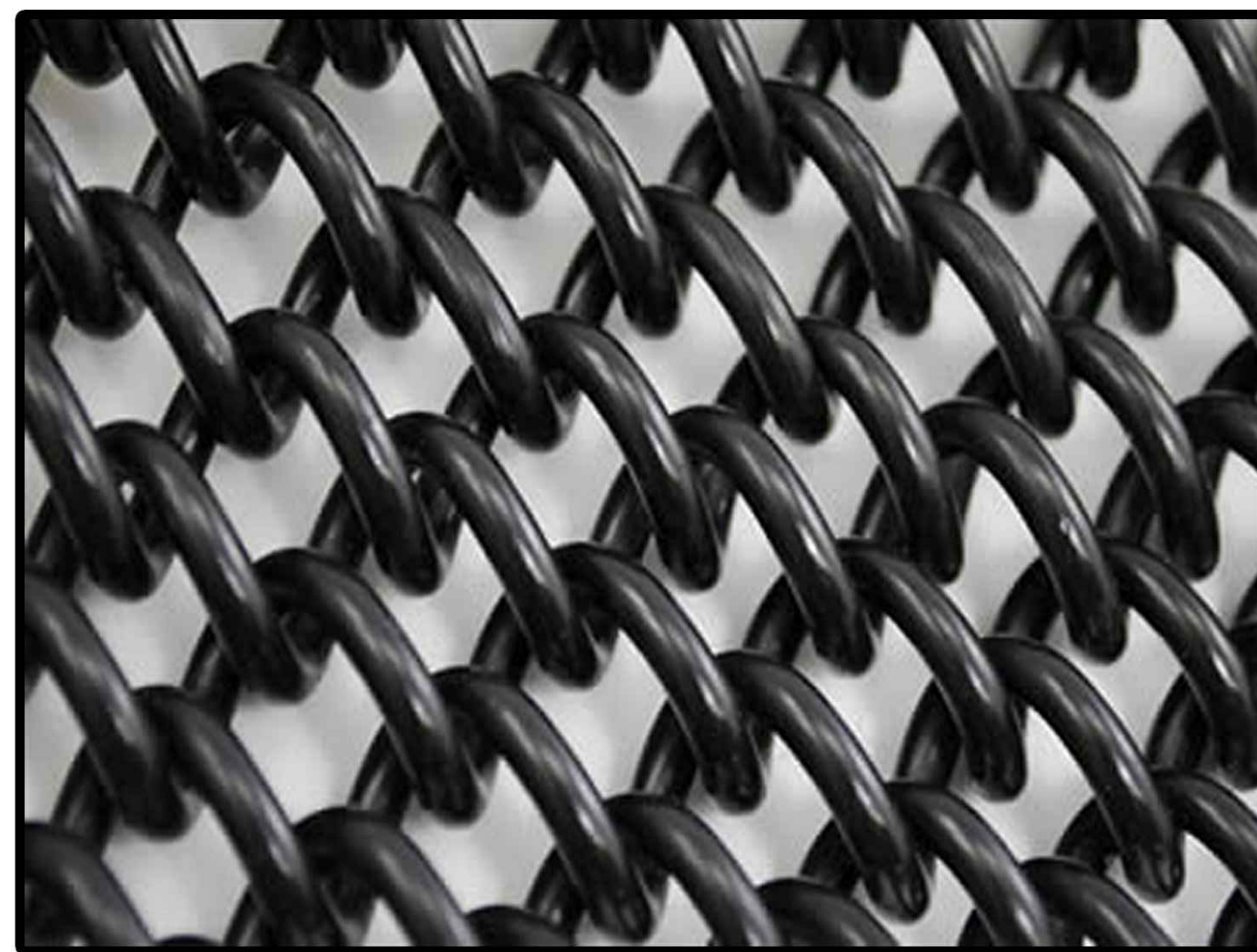
FENCE: 11 GA. X 3/8" BLACK VINYL COATED GALVANIZED SECURITY MESH FRAMING TO HAVE DIRECT TO METAL COATING THAT MATCHES SECURITY MESH
